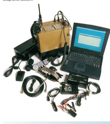
Channel scanning combined with the "Selcall Option" means calls will always get through, no matter what frequency or channel is operational due to propagation. Two scan tables are available, channels can be programmed as members of either table or both.
